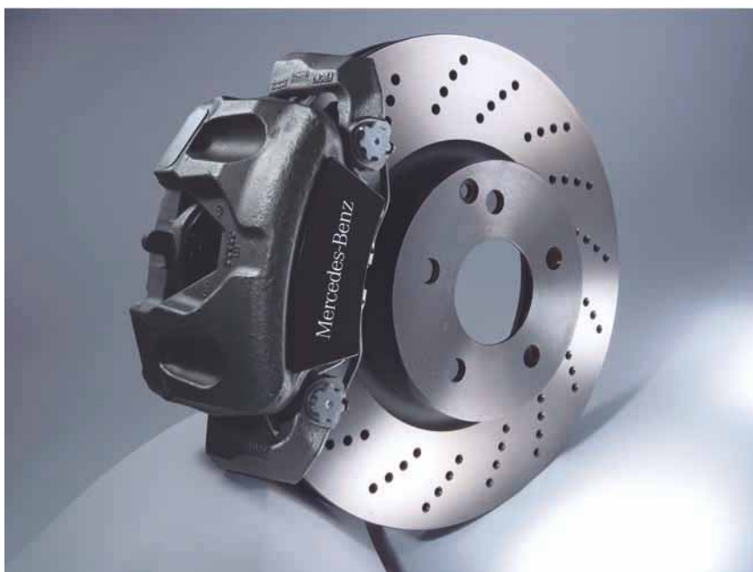
Front brake disk, perforated with aluminum composite brake caliper and Mercedes-Benz lettering (sports version)
